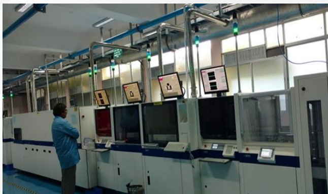
Automated In-line Metalisation (Screen Printing) Stations of Solar Cell Manufacturing Facility
